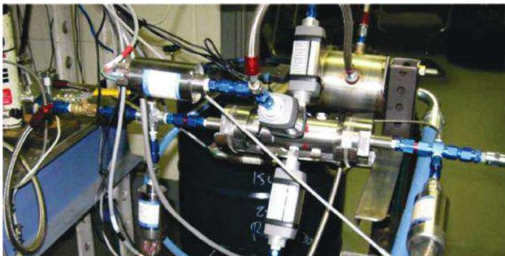
Application of a device with a working diameter of 25 mm and a capacity of 250 litres per hour in the preparation of a gasified fuel composite (from No. 2 diesel and compressed air).
