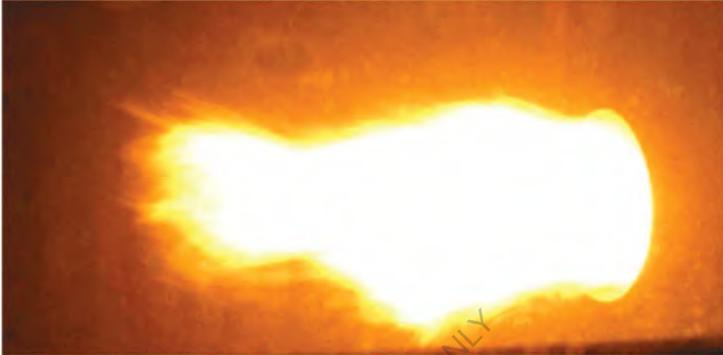
Shape of the flame when using as fuel, - diesel fuel #4, mixed online with water (20% by weight) and compressed air (3% of stoichiometric proportion, pressure 5-6 bar); Flame volume increased, flame temperature 25% higher, sharp reduction in soot, carbon, carbon monoxide and nitrogen oxides.
