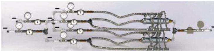
**Figure 2.** - The figure shows a system for feeding, metering and on-line preparation of different fuel mix variants, consisting of a number of independent parts and components.
