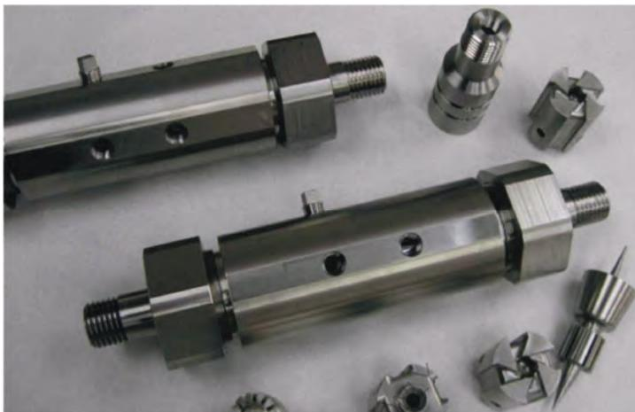
A device for dynamic mixing and homogenisation of liquid fuels and fuel mixtures and for the formation of gasified (compressible) fuel mixtures . The pictures show a device with a working diameter of 40 mm and a capacity of 1000 litres per hour.
