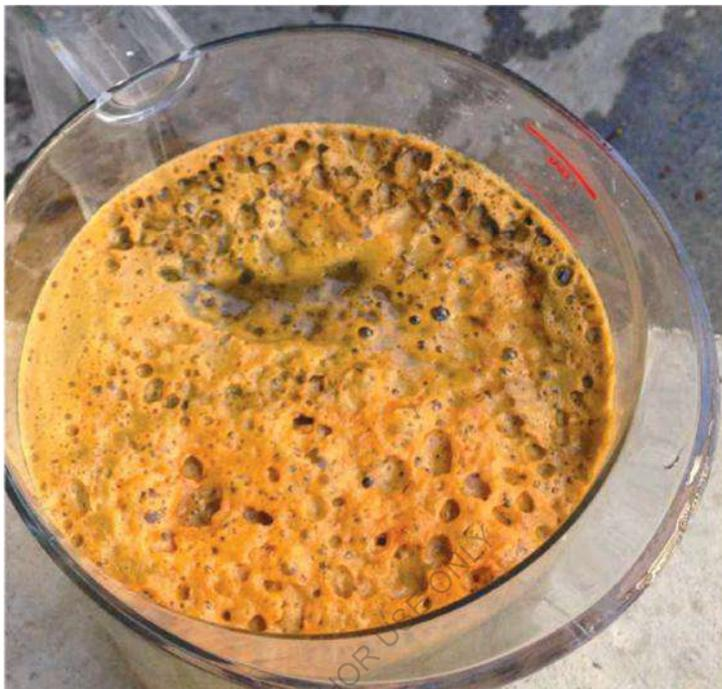
The image shows a foam layer produced by a foam generator in the wastewater of a modern butter production facility.
