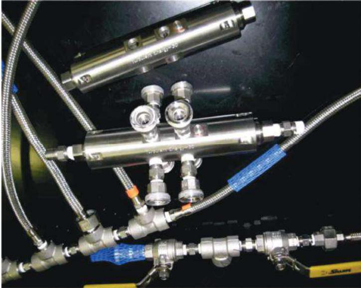
Devices with a working diameter of 30 mm; Devices can be manufactured on commercially available numerically controlled machine tools without the need for special metal-cutting tools; All connections, piping and sub-assemblies are made from standard parts; All piping includes all necessary parts, fittings and piping components;
