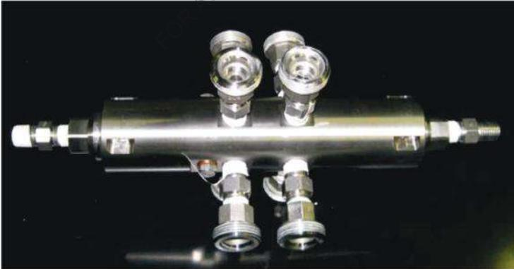
Experimental device for mixing fuel mixture components; Especially flexible hoses are used in the system; The device has extremely small dimensions; The capacity of the device, - 150 litres of fuel mixture or emulsion per hour.
