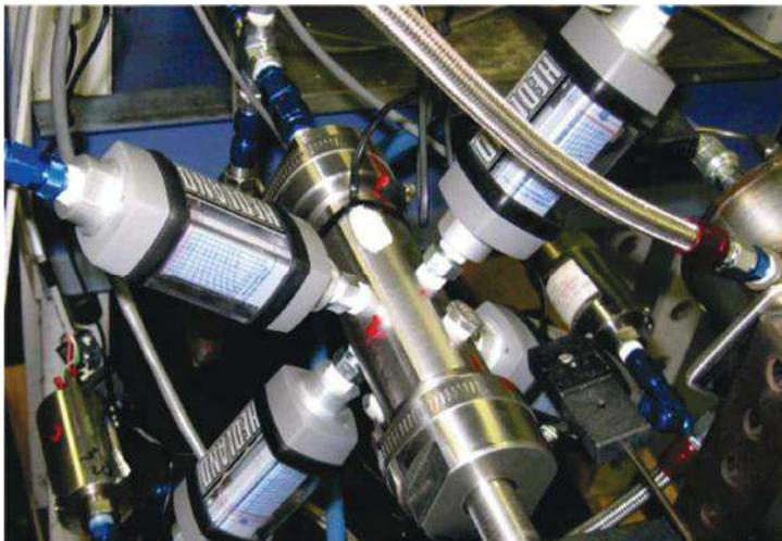
Application of a device with a working diameter of 25 mm and a capacity of 250 litres per hour in the preparation of a gasified fuel composite (from No. 2 diesel and compressed air).
