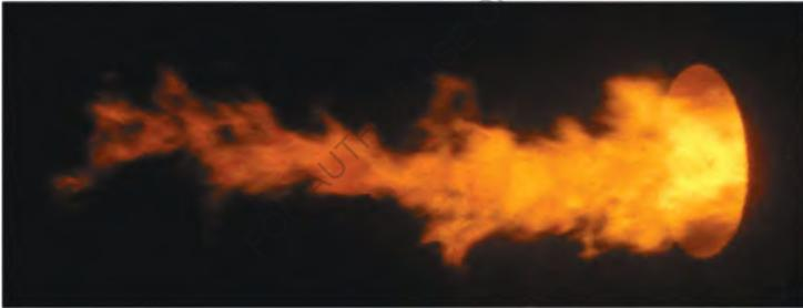
Flame pattern when using normal fuel for this burner - diesel No.4 ; Fuel flow rate, fuel line pressure, type nozzles, air flow rate, air flow pressure are completely identical for all tests.
