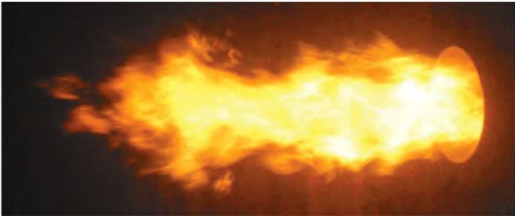
Shape of the flame when using as fuel, - diesel fuel #4, mixed online with water (tap water, 15% by weight) and compressed air (3% of stoichiometric proportion, pressure 5-6 bar); Flame volume increased, flame temperature 20% higher, sharp reduction in soot, carbon, carbon monoxide and nitrogen oxides.
