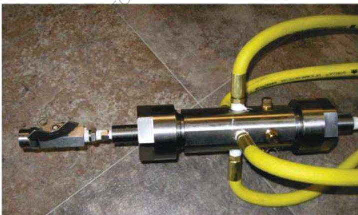
**Figure 4 - 2**, - the figure shows a fragment of the system made in stainless steel. The system is designed to homogenise milk at low pressure (standard systems homogenise at extremely high pressure).
